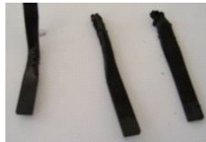
Plain SLS UL94 Burn Test - Failed
