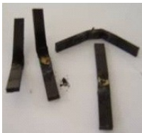
RP Tempered FDM 5VA - Passed
