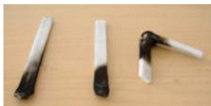
Plain FDM UL94 Burn Test - Failed
