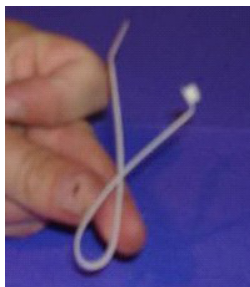
RP Tempered™ FDM Living Hinge Completed 50 Cycles without Breaking
