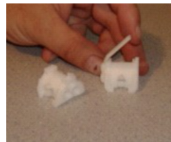
RP Tempered™ FDM Living Hinge Completed 50 Cycles without Breaking
