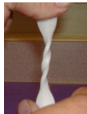
RP Tempered™ FDM Tensile Bar Bends and Twists Without Fracturing
