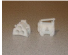
RP Tempered™ FDM Living Hinge Completed 50 Cycles without Breaking
