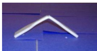
Plain FDM Tensile Bar Fractured at 1/2 Bend
