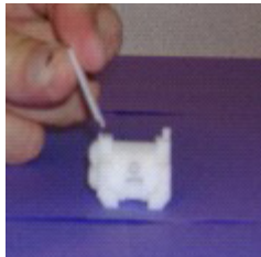
Plain FDM Living Hinge Part Fractured on First Cycle
